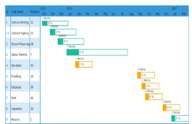
The progress of the construction activity is shown by shading the bar with colour or hatching. *Note:* The disadvantages of Gantt Chart are:
